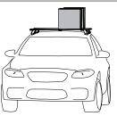
120kg/264lbs load rating (Urban road) **80kg/176lbs load rating** (Off road - 120kg / 1.5)
